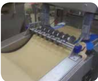
Strip cutting on the inlet conveyor
